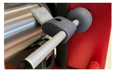
An anvil surface free of wear is an important factor for successful die-cutting. Wear on the anvil may cause die-cutting issues and shorten the life of your dies. Proper cleaning and lubrication are critical to prevent these issues and keep your anvils in top condition.
