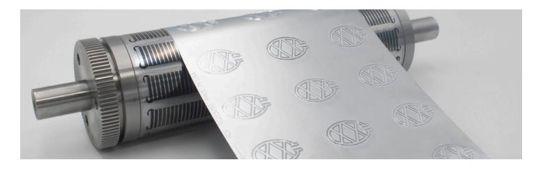
**FLEXIBLE DIES** are an excellent cost-effective option for cutting thin material such as paper and film. However, flexible dies tend to have a shorter useful life than solid. To maximize the life of your flexible dies, proper maintenance is key. Here are a few best practices to keep your flexible tooling cutting properly for the longest possible time.
