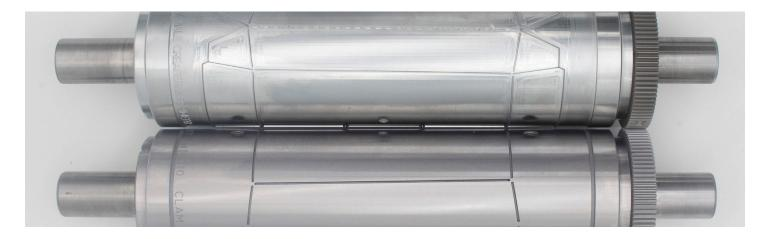
Creasing is generally used to fold a material. There are three very different types of creases (Crush, Cut, and Male-Female). Each one is used on specific materials or applications.
